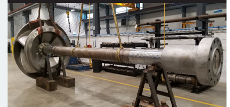
Rotor assembled and ready for balancing
