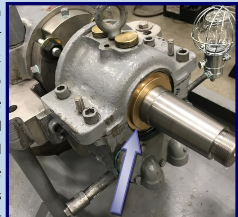
Isolator Installed in Split Bearing Housing
