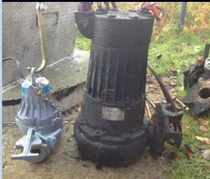
tested side by side to compare results. The Flygt pump was pulled monthly and checked for debris in the volute. It was clog free & clean every time.
