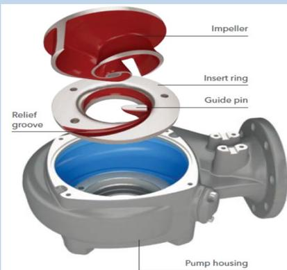
impeller design introduced in early 1999. The N impeller design has proven itself over the last 16 years to be the best impeller design for eliminating clogs. The screw shaped impeller with beveled edges self cleans itself against a relieve groove after each revolution, eliminating modern trash from being hung up on the impeller. This design
