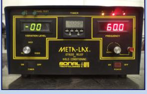
Through sub-harmonic vibrations, produced by the Meta-Lax machine, weld distortion, porosity, and internal stresses are greatly reduced during the weld process. It also improves fatigue life, weld ductility, uniform weld grain among other key factors in fabrication. Customers will now receive reconditioned or fabricated parts with higher quality welds and receive decreased lead times.
