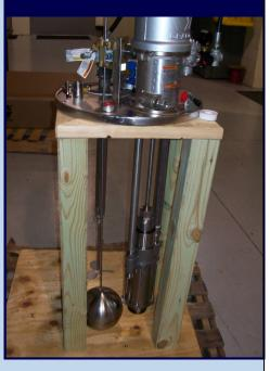
the tank is full the plant needed to turn on the air operated pump to transfer the used solvent to a larger holding tank outside the plant. The plant did not want to use an electrical level sensor
