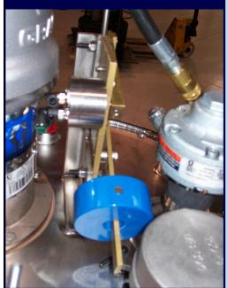
Problem: A Chicago Area Automotive Final Assembly plant wanted a float control valve that could control their air operated solvent recovery. The plant wanted to turn an air operated pump on and off with using an expensive explosion proof level sensor.
